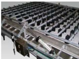
Individually adjustable UHMW polyethylene plows are free floating but properly weighted to always maintain contact with the belt. More rows and more plows increase belt exposure to allow filtrate to escape.
