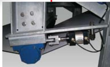
CMC utilizes a pneumatically controlled center pivot alignment system. This design reduces belt stretching, lengthens belt life and provides a more consistent performance over the life of the belt.
